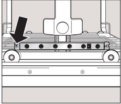
■ Place the track in the holder of the mobile unit and screw firmly in place.
